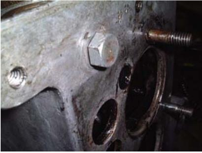
Screw fully home allowing for fibre washer
