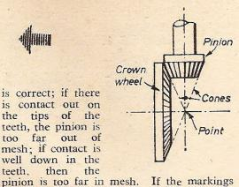
are on one side at one end and on the other side at the other end, then the pinion has to be moved and the crown wheel adjusted to suit. In your circumstances, we suggest you try various combinations of shims, inserting and removing some, and adjusting the crown wheel by means of the threaded rings either side.
