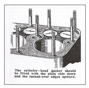
You should, however, try the cylinder-head nuts again after you have run the car for a few days, as usually they can be taken up slightly, the gasket having bedded down meanwhile.
