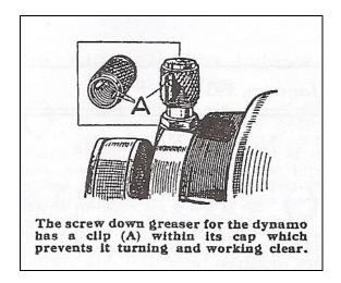
Further, if they are well packed with the stiff grease recommended for the points concerned, this grease will also help to keep the caps from working off, and when they are screwed on sufficiently to be secure there should be several turns available for pushing the grease to the bearings concerned, before the cap will need replenishing.
