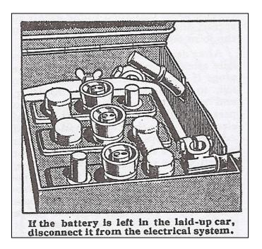
Usually the battery should then last a very long period if in reasonably good condition to start with. Alternatively, you could charge the battery and drain it of electrolyte (i.e. acid) and wash it out with distilled water, this policy being adopted to avoid sulphation of the plates. The battery should then remain in good condition for some time. It should not be connected to the electrical circuit of the car.
