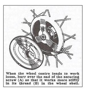
**A.** The securing screw beds in a taper seating in the wheel centre, and you should ensure that both the screw head and the taper are clean to make a sure grip. Dirt at this point might result in the screw working loose. In any event, if you burr over the end of the screw just sufficiently to make it somewhat stiff to turn in its thread, this extra resistance should prevent the screw and plate from working loose.
