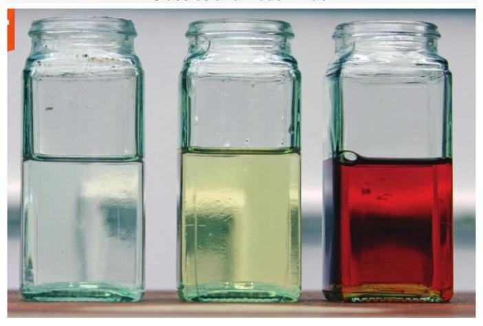
Much has been written about modern fuels and their ethanol content, but the above picture provides visible proof that it degrades. The jar on the left contains fresh petrol, the middle one is a few months old and the one on the right has been in a tank for many years. The issue affects carburettor fed engines far more than fuel injection cars.
