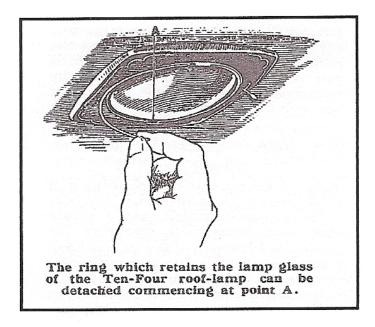
Access to the bulb is very easily gained. The frosted glass of this lamp is held in by a wire ring which fits in two tangs formed inside the lamp frame. By carefully springing one end of the ring clear of the tang, and then releasing the ring from the other side, the glass will come clear, although it may need easing carefully past the tangs just mentioned. The bulb is then accessible, being mounted in a normal bayonet socket. It is the same as those used for the rear and side lamps.
