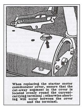
This as you found, will cause erratic operation and overheating of the starter switch. When you replaced the cover and switch on your starter for the second time, you must have positioned the cover correctly, which explains why the starter afterwards worked satisfactorily.
