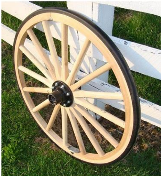
The next development – a solid rubber tyre.
