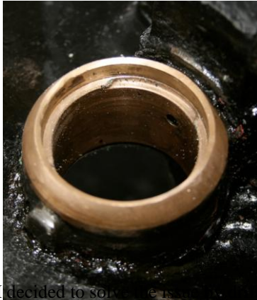
Fig 2 - showing wear in stub axle collar.
