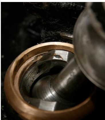
Fig 1 – The Ball and Pin 'UJ' in the stub axle assembly
