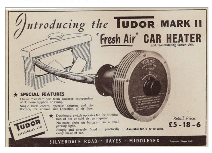
This seems like a simple heater system, no breaking into the coolant system and also suitable for cars without a water-pump, pity these heaters are not available today.
