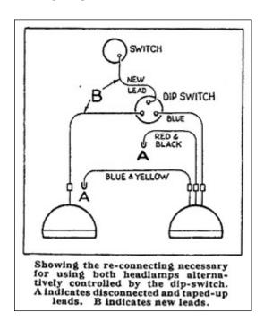
The circuit could be revised to permit either headlamp to be used at will in the following manner:
