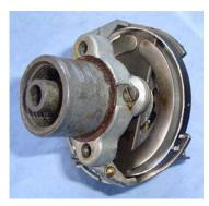
v. Check how freely the pawl arm moves in its groove; if it is stiff the groove needs filing. Check the profile of the arm at point of engagement.
