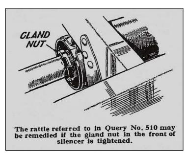
One point which may definitely repay examination is the gland nut at the front of the silencer. This, after a period of usage, may have worked loose, to rattle on the exhaust pipe, in which event, by tightening this nut well home you will stop the noise you are experiencing.
