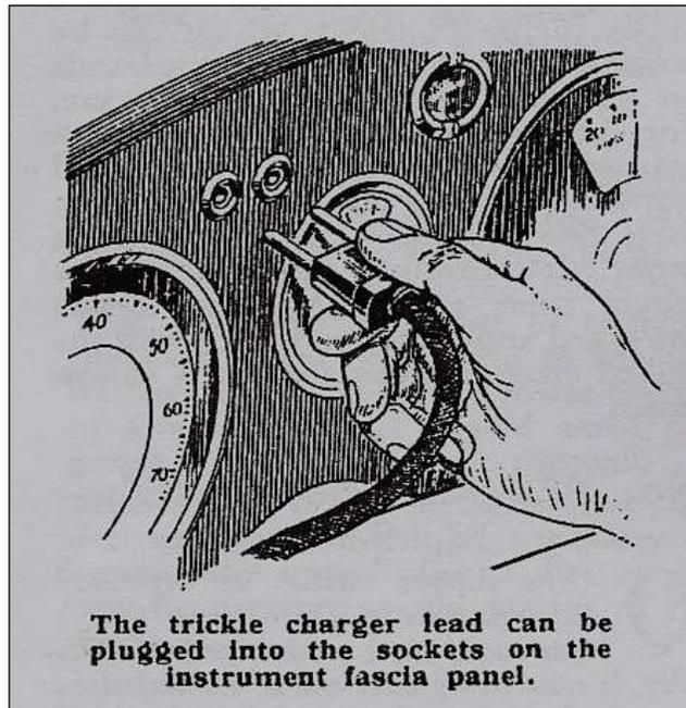
The red terminal is the positive which is earthed, and when fitting the charger care should be taken to connect the corresponding terminals accordingly. Suitable plugs to fit the pin sockets can be easily cheaply obtained at almost any radio store.
