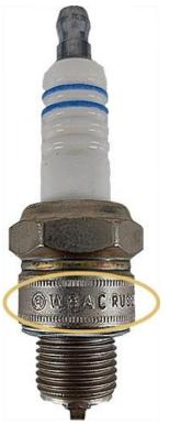
Cool Air stock two brands of spark plugs, Bosch and NGK. Using the first few letters and numbers on a spark plug we can ascertain what size, length and heat rating it is.
