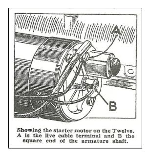
This is located close to the squared end of the armature but it should be possible to turn the latter without making such contact. However, if you have occasion to release the starter pinion in this way you might prefer to cut off the electric current by disconnecting the cable from the negative terminal on the battery to be found under the front passenger's seat.
