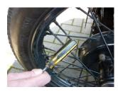
should give a nice melodic twang (outer) or ping (inner). If not, get tightening. Rust at the hub is a clue. Oh, and don't forget the spare wheel. Check the BACK of the tyres for cuts, cracks and damage. Then have a second look at the outside and the tread. Plenty left, no cracks, nice and even please. Wheel nuts tight but not barmy, do not use an extension bar on a socket.
