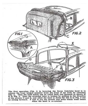
**A.** To lower the roof on your Austin Pearl cabriolet the following procedure should be adopted: Release the two fastenings above the windscreen (one is shown at A in Fig. 1) and lift the canopy rod. Then detach the three clips which secure the front bar
