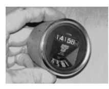
The Lucas Magmo speedometer was used on Austin Sevens from 1932 to 1935. My repair became necessary because the rotating speed reading dial was stuck at the near zero position and only a sharp tap of the hand whilst driving would make the dial free to move. It would then work fine until the next prolonged stop.
