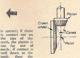
pinion is too far in mesh. If the markings are on one side at one end and on the other side at the other end, then the pinion has to be moved and the crown wheel adjusted to suit. In your circumstances, we suggest you try various combinations of shims, inserting and removing some, and adjusting the crown wheel by means of the threaded rings either side.
