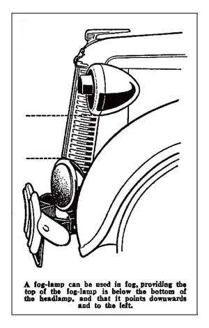
The fog-lamp must be operated by a separate switch; its light must be directed downward and to the left; and in the event of an air raid warning it must be extinguished. You can also use an unmasked headlamp in fog, as a substitute for a fog-lamp, if the foregoing conditions are complied with (excepting, obviously, that the fog-lamp location), and providing not more than one authorized masked headlamp is in use at the same time.
