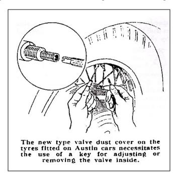
On removing the dust cover this key can be inserted into the valve for its slotted end to engage with the valve-inside to unscrew or adjust the seating of the latter as may be required.
