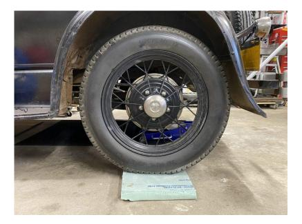
Tyres are made for driving, not for parking. That's why long-term storage is likely to cause flat spots or dry-rotting of the rubber rings we need so dearly. There are appropriate products on the market that can help, but it's also just as easy to pick up some insulation foam board and cut a few squares that fit under your tyres. This will form a cradle for the tyre and also keep the dirt or concrete under the car from sucking the moisture out of the rubber, making them last longer.
