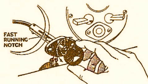
Showing the fast engine running position of the strangler control on the Twelve-Six.
