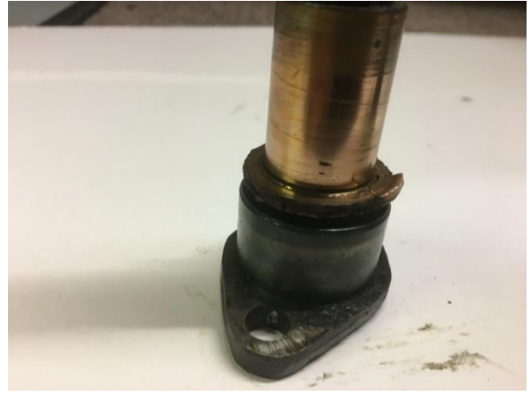
The 'disintegrating' layshaft bush
